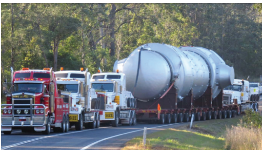
(b) Heat exchanger delivery from Coffs Harbour to Olympic Dam: 2400 hp from 4 prime movers towing 358 tonnes 2250 km
