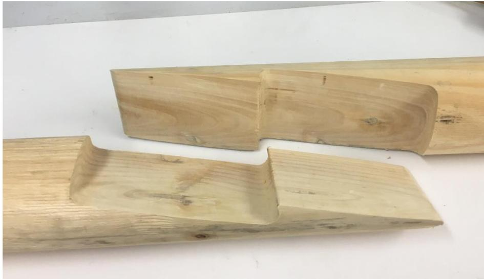
**CNC routed Hooked scarf Joint**
