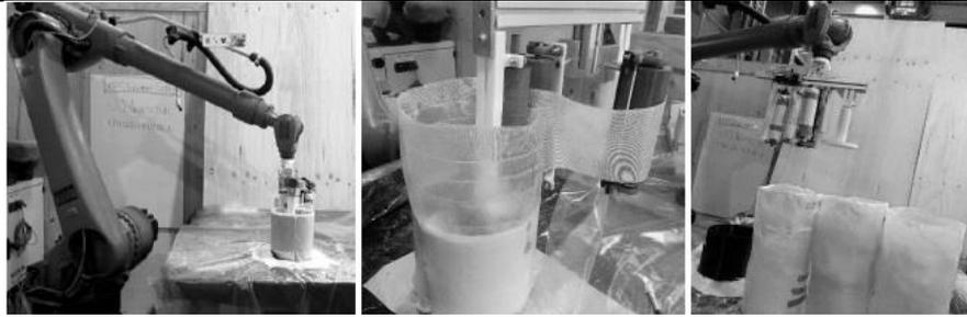
Figure 2 Robotic FRP formwork fabrication
